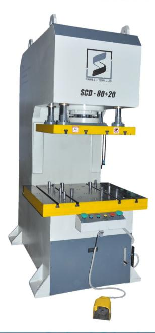
The C-frame press derives its name from the shape of the frame. The primary advantages to the C-frame design are an open work area and increased accessibility. The C-frame press features become even more advantageous when multiple presses are used for progressive operations with automated material handling moving parts from press to press. The C-Frame hydraulic presses, however, are generally limited in maximum tonnage due to the design.
